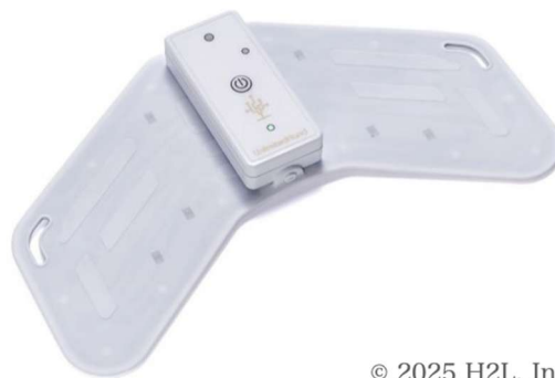
Figure 4-20 “UnlimitedHand” by H2L, equipped with an output mechanism of proprioception by electric stimulation in addition to muscle displacement sensor
