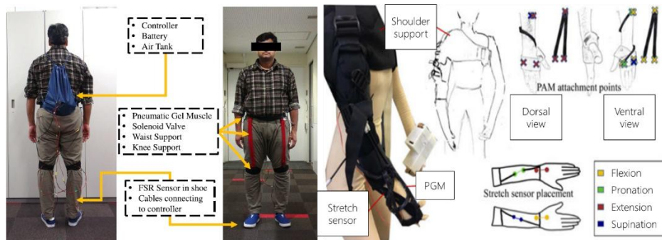
Figure 4-3 Examples of utilizing artificial muscles for gait support (left) and upper limb movement support (right)
